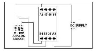
If no 0 – 10V sensor is available use none, one and then two (in series) AA batteries across B1 and B2 terminals in the tests below.
